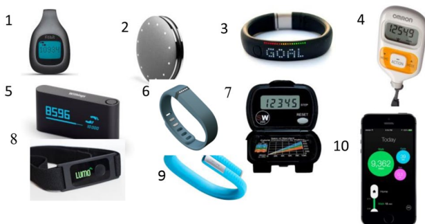
Figuur 1 Tien activity trackers die werden getoetst op hun accuratesse. 1 Fitbit Zip, 2 Misfit Shine, 3 Nike + Fuelband, 4 Omron Walking style III, 5 Withings Pulse, 6 Fitbit Flex, 7 Digiwalker SW-200, 8 Lumoback, 9 Jawbone Up, 10 Moves app.
